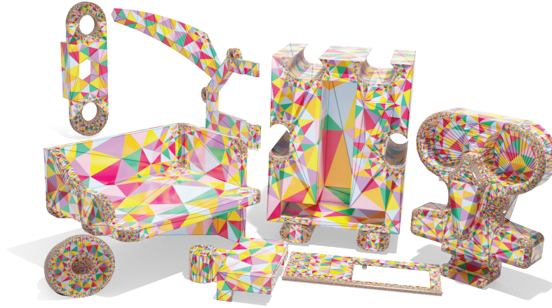
Figure 3.9: Intrinsic Delaunay refinement inserts new vertices intrinsically into a mesh to improve the triangle quality. We show that (under a few assumptions), intrinsic Delaunay refinement is guaranteed to produce a mesh whose triangles all have corner angles of at least 30^\circ .
